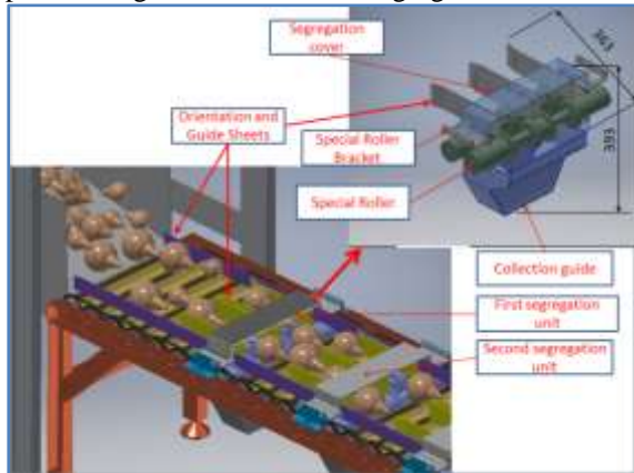
Figure 15, Segregation unit isometric view
